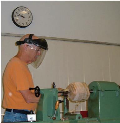
Step 1: Properly select and prepare your blank. Pay attention to grain direction and future shrinkage. Mount between centers top to headstock.
