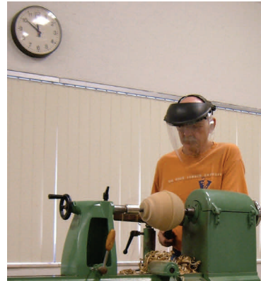
Step 2: Rough turn the outside shape. Make a proper tenon that will fit your chuck exactly. Leave stock above the tenon to finish the bottom curve.
