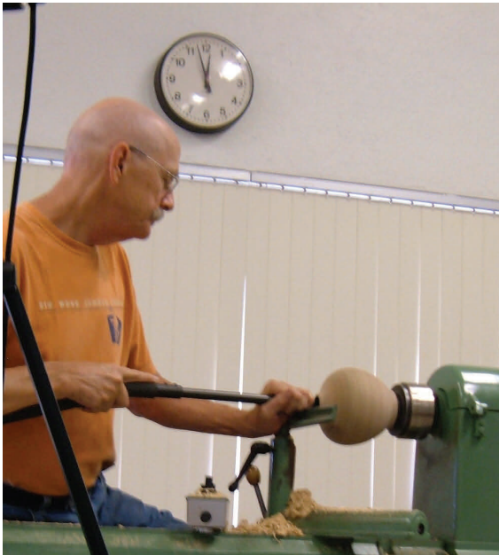
Step 4: Drill the vessel to full depth and begin hollowing with a 3/16" straight tool.
