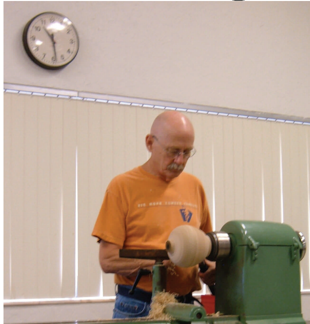
Step 3: Mount the vessel in the chuck and refine the outside shape. Finishing the outside by shear scraping with the gouge and scraper.
