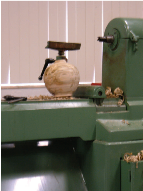
The roughed vessel with a completed tenon is ready for the chuck.
